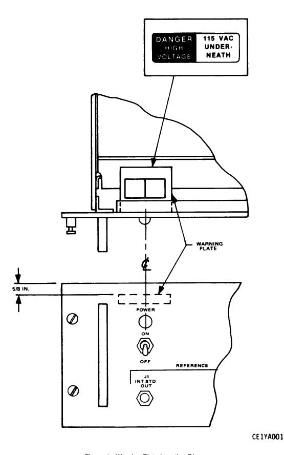
Figure 1. Warning Plate Location Diagram
